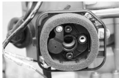
1. Set the starting lever (choke) to the
